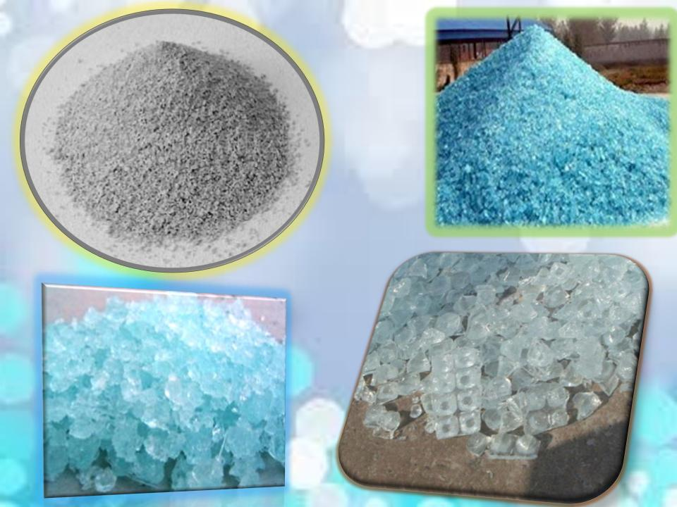
Varying the proportions of SiO2 to Na2O and the solids content results in solutions with differing properties that have many diversified industrial applications. These are sold as 20% to 50% aqueous solutions called water glass.
