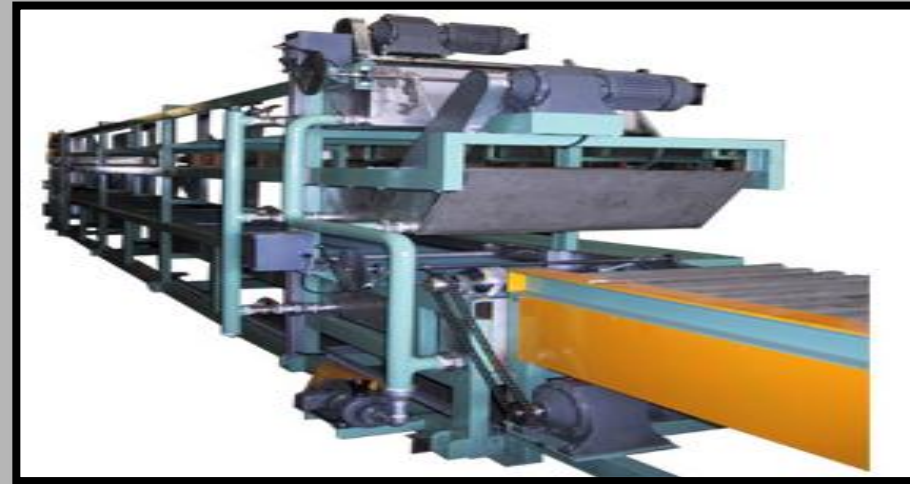
TYRE TREAD COOLING EQUIPMENT
