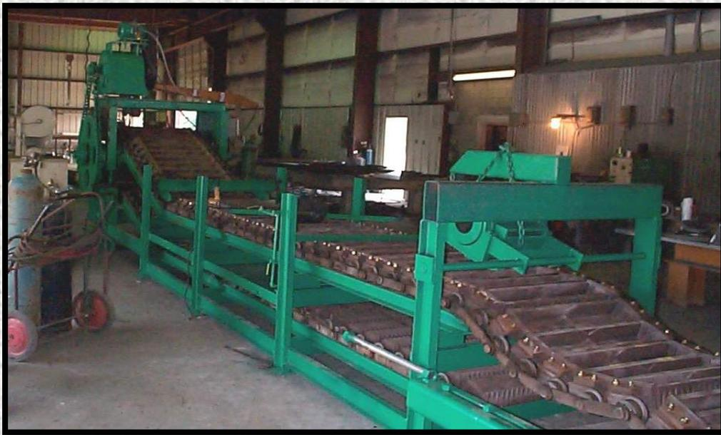
**INGOT CASTING ROTARY CONVEYOR**
