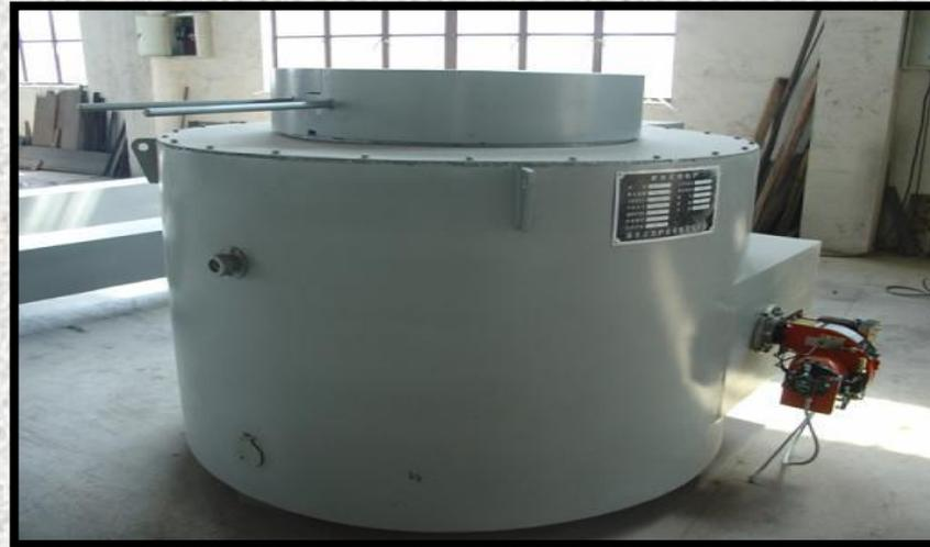
**ALUMINIUM MELTING HYDRAULIC CRUCIBLE FURNACE**
