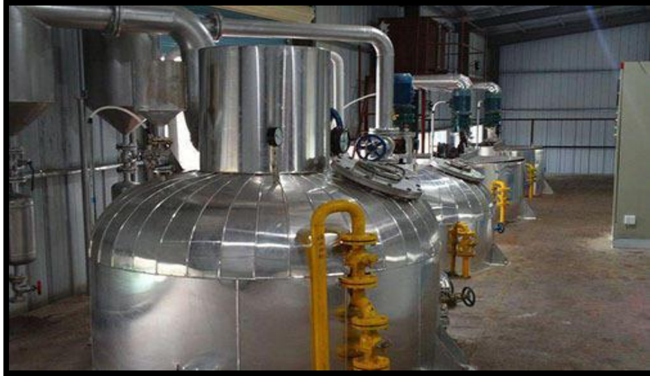
Continuous Deodorizing Section
