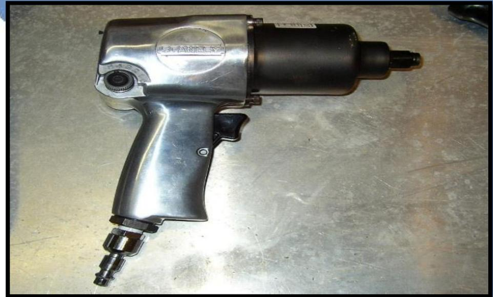
**Screw, Nut, Bolt Tightening Machine**
