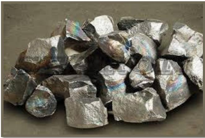
**Ferromanganese is a ferroalloy that has high content of manganese; it is manufactured by heating mixture of oxides  $\text{Fe}_2\text{O}_3$  and  $\text{MnO}_2$  along with carbon, which is usually coke and coal in an electric arc furnace or blast furnace. In the furnace, the oxides go through carbothermal reduction, hence, producing ferromanganese which is used as deoxidizer for steel. Main producing countries of Ferro Manganese are India, South Africa, Korea & Europe.**
