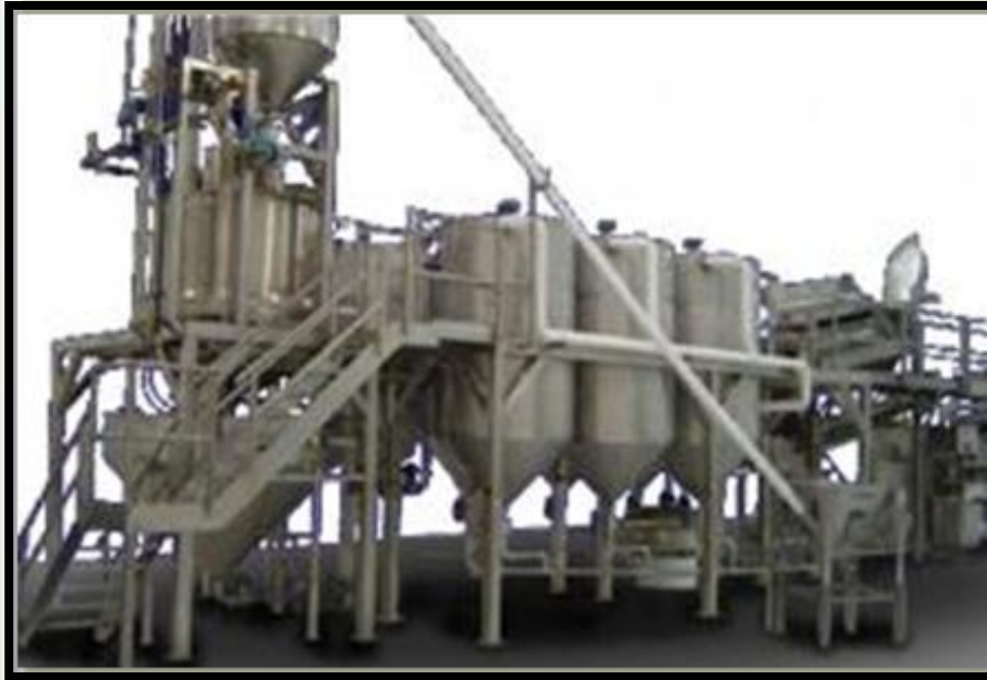
Steeping – Steeping System
