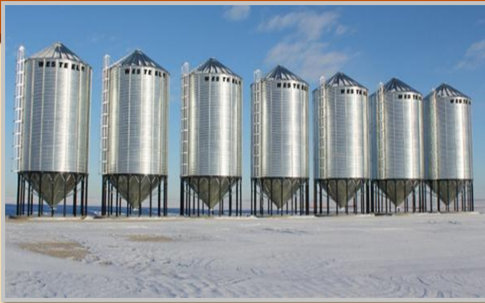
Batching System (Over ground Frame & Ram Material Silo)
