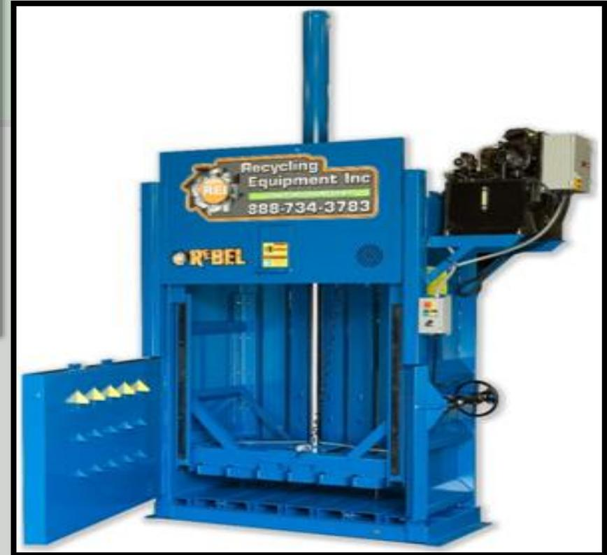
**Electrically Operated Vertical Type Bailing Machine**
