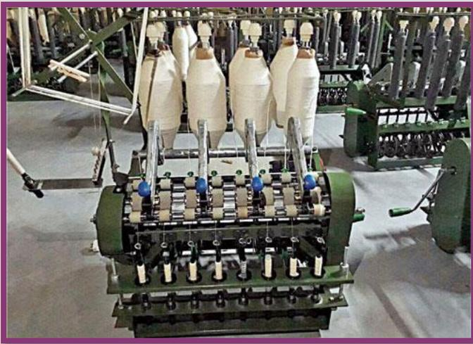
**Yarn from a solar charkha are stronger compared to the manually operated charkha. In fact yarns of desired strength could be achieved by proper choice of the drive. Yarn are more uniform compared to a manually operated. This is because of the incorporation of a battery which helps to give uniform power even in the variable climatic conditions.**
