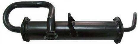
**The noise of the burning-hot exhaust gas exiting the engine at high velocity is abated by a series of passages and chambers lined with roving fiberglass insulation and/or resonating chambers harmonically tuned to cause destructive interference, wherein opposite sound waves cancel each other out.**
