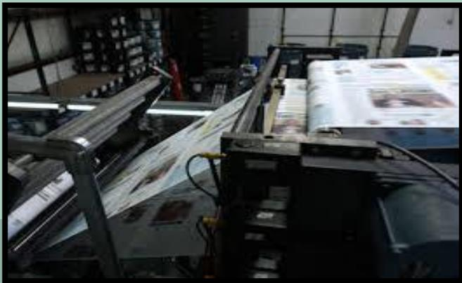
**Web offset printing is a type of offset printing that continuously feeds a roll of paper through the press. The paper is not precut but is after the printing is complete and then goes to bind or fold. Web offset presses are able to print on one or two sides simultaneously. With these features, web offset printing is perfect for those larger commercial projects. Web Offset printing is one of two variations of offset printing; the other being sheet-fed offset printing.**
